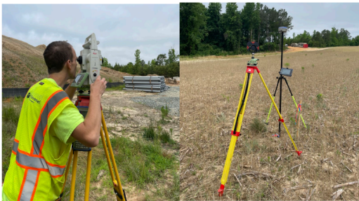
Figure 3: Total station operation (left), Back-site (right image shown on a yellow tripod), GPS shown on right image as black pole with tablet and round antenna
